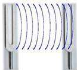
Figure 5. Light scattering and tuning forks. A vibrating tuning fork causes in air between it and another tuning fork to vibrate, which in turn causes the second tuning fork to vibrate. The analogous behavior with electromagnetic radiation is the emission of light from oscillating electrons in matter, the light is later scattered by electrons surrounding an atom or molecule at another location.
