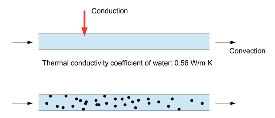
Thermal conductivity coefficient of magnetite ( $Fe_3O_4$ ): ~1 W/m K
