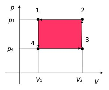
$$W = p_4 (V_2-V_1) + p_1 (V_1-V_2) > 0$$
