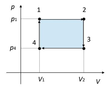
$$W = p_1 (V_2-V_1) + p_4 (V_1-V_2) > 0$$
