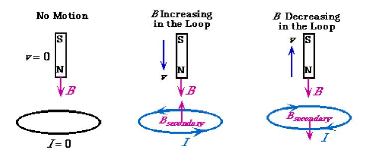
**Lenz's Law**: emf will be produced when the magnetic flux is changing as function of time.
