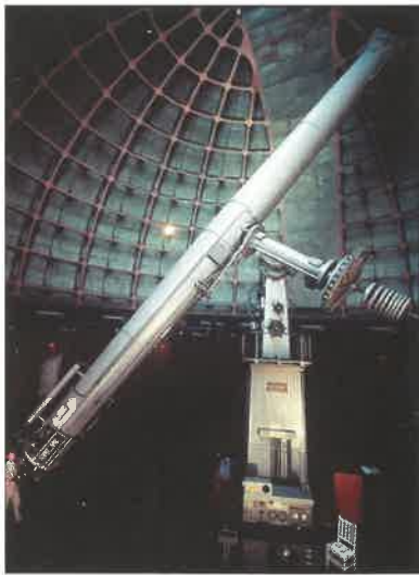
Figure 2.4 The 36 inch refractor at the Lick Observatory, California. (© UCO/Lick Observatory)
