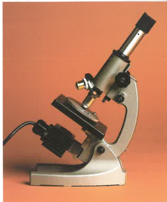
Figure 8.1 A simple petrographic microscope (or polarizing microscope).
