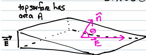
$$\text{flux through top surface is } \phi = EA \cos \theta = \vec{E} \cdot \vec{A}$$
