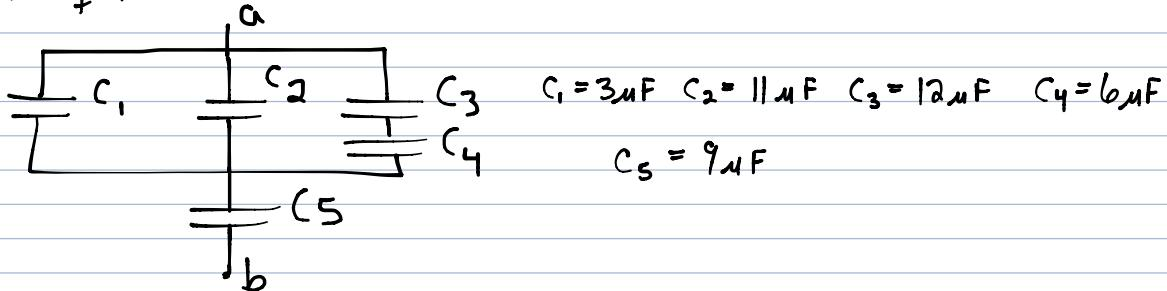
$$C_{eq} = \frac{C_1 C_2}{C_1 + C_2} + C_3 + C_4 + C_5$$
