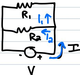
$$V = V_1 = V_2 \text{ and } I = I_1 + I_2 \Rightarrow \frac{V}{R_{\text{req}}} = \frac{V}{R_1} + \frac{V}{R_2} \Rightarrow \frac{1}{R_{\text{req}}} = \frac{1}{R_1} + \frac{1}{R_2}$$
