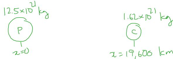
$$A) x_{cm} = \frac{\sum x_i m_i}{\sum m_i} = \frac{(0)(12.5 \times 10^{21} \text{ kg}) + (19,600 \text{ km})(1.62 \times 10^{21} \text{ kg})}{12.5 \times 10^{21} \text{ kg} + 1.62 \times 10^{21} \text{ kg}}$$
