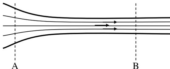
Speed is higher at B, so according to Bernoulli's law, the pressure is lower at B.
