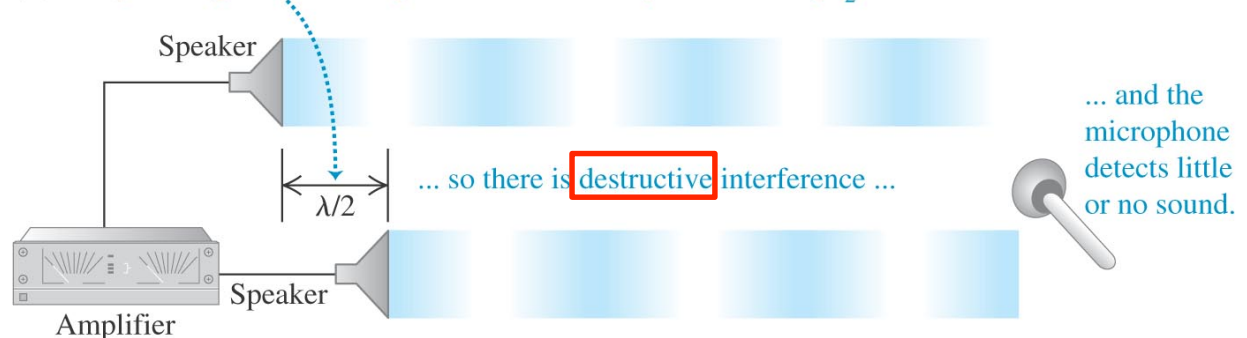
(b) The path lengths from the speakers to the microphone differ by \frac{\lambda}{2} ...
