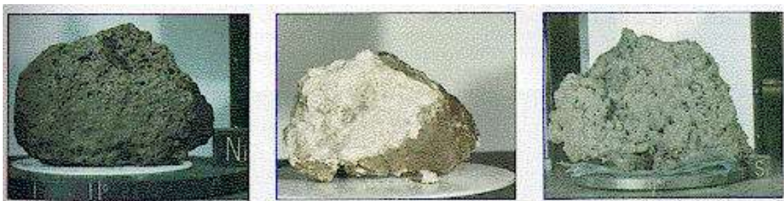
Figure 8. The three major types of moon rocks. Panel A. A dark mare basalt. A 1-cm block is shown for scale. Panel B. A highlands anorthosite. Panel C. A gray and white breccia. P 149-8.8&8.9&8.10.
