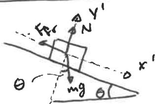
$$\frac{x'}{mg \sin \theta - F_r = ma_x} \quad \text{--- (1)} \quad \frac{y'}{N - mg \cos \theta = 0} \quad \text{--- (2)}$$
