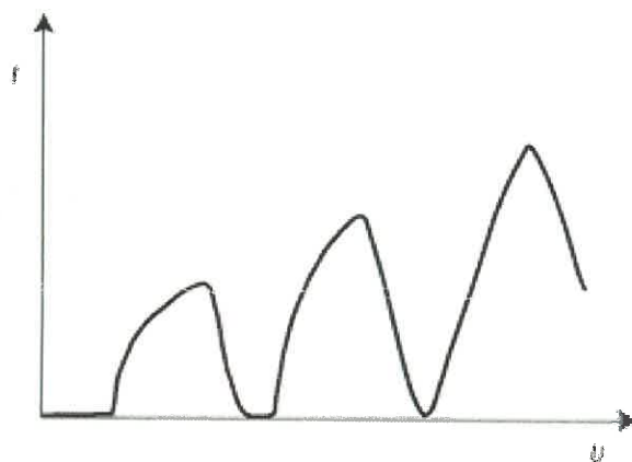
Fig. 3 Target current I as a function of the accelerating voltage U
