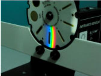
5. Rotate the scanning arm until it touches the stop. This will be the starting position for all the scans.
