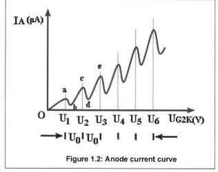
As a matter of fact, a strong line can be found for emission and absorption corresponding to an energy of e•U<sub>0</sub>, the excitation energy of argon, in the optical spectrum (108.1 nm).
