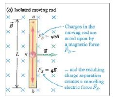
• For a closed conducting loop moving (with velocity  $\vec{v}$ ) in a magnetic field,  $\vec{B}$ , the induced emf could be calculated as
