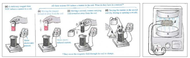
• The direction of the induced emf (or induced current) could be determined Lenz's Law. (the direction of the induced current is as if the system is trying to maintain the original magnetic status; or equivalently, the direction of any magnetic induction effect is such as to oppose the cause of the effect.)
